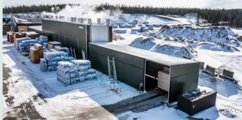
Valutec's timber dryers at Kåge sawmill.
